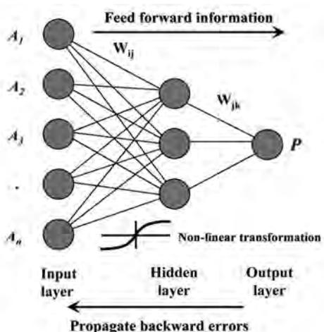
Figure 1 : Architecture of Multi-layers perceptron.
