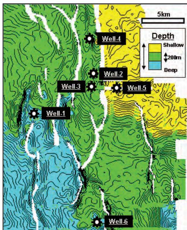
Figure 2: Depth structure map of top Z-sand Reservoir in the study area.
