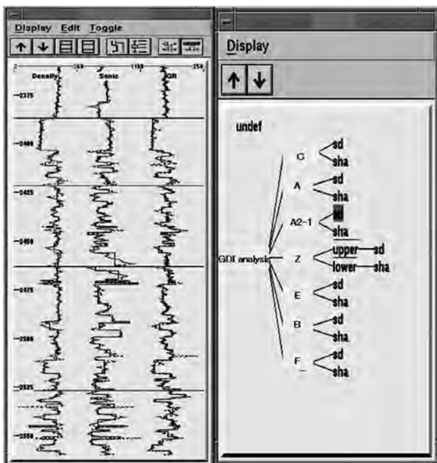
**Figure 4:** Geological-stratigraphic model established from real geological information including well logs, stratigraphic sequence, lithologic units and geological knowledge.
