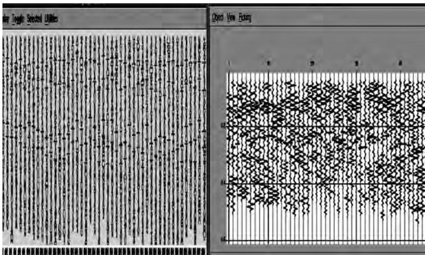
**Figure 5:** Part of pseudo wells (left) generated by Monte Carlo simulation and corresponding synthetic traces (right), based on the geological-stratigraphic model.
