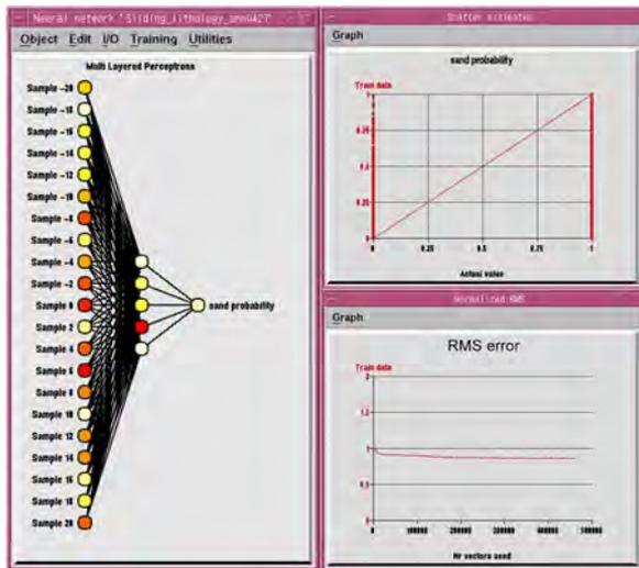
**Figure 7:** The trained ANN (left) and its performances (right) for establishing the relationship between the lithologic code and seismic attributes. Nodes are displayed in color scale relative to their contribution to the output, i.e., from red (highest), orange, yellow to white (lowest).
