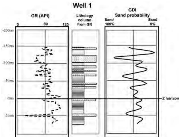
Figure 11: Comparison of predicted lithology by GDI with GR from factual well 1 at well locations. (Solid line: sand probability, Dotted line: GR).
