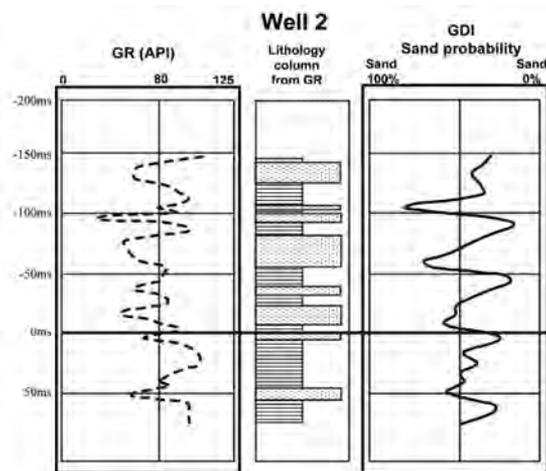
Figure 12: Comparison of predicted lithology by GDI with GR from factual well 2 at well locations. (Solid line: sand probability, Dotted line: GR).
