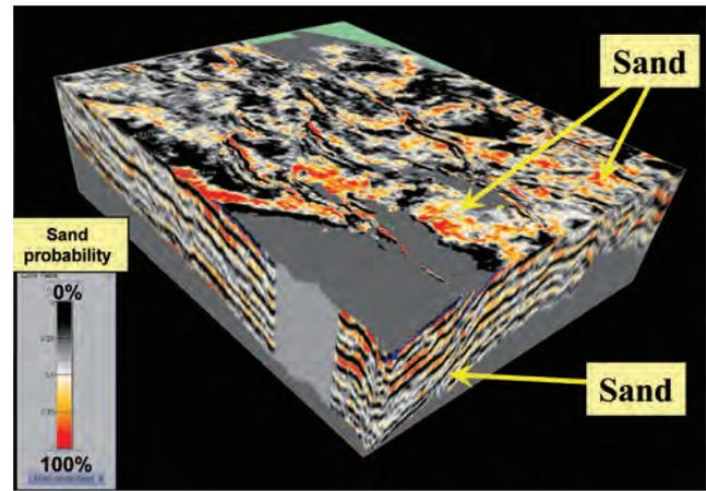
**Figure 8:** A lithology cube created by applying the ANN to 3D seismic volume. It shows the distribution of sand probability from A horizon to B horizon within the seismic volume.
