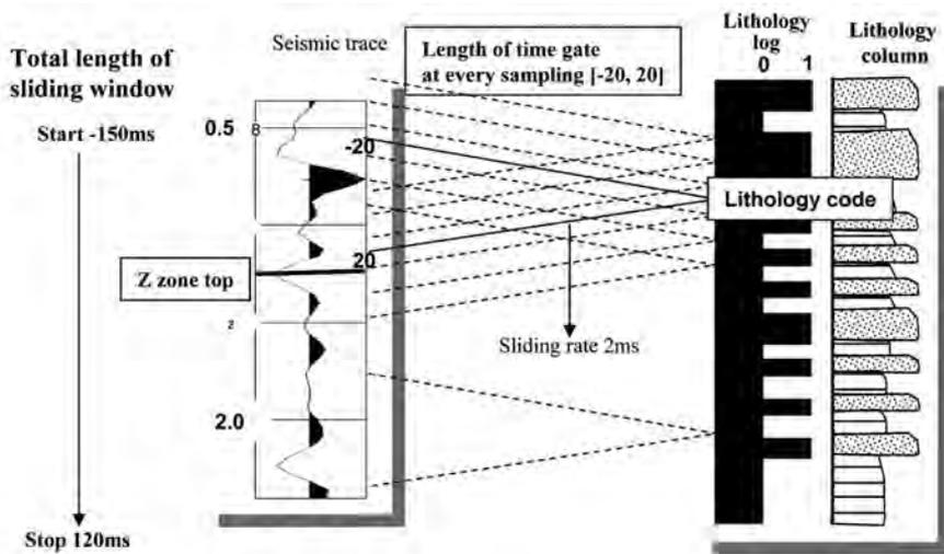
**Figure 6:** Lithology extraction from pseudo wells and seismic attributes (Sample or Amplitude) from synthetic traces as known samples.
