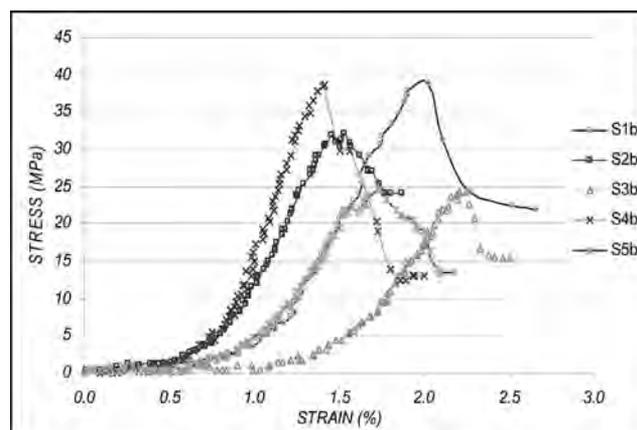
**Figure 7:** Stress-strain curve for sandstone tested under servo-controlled machine.
