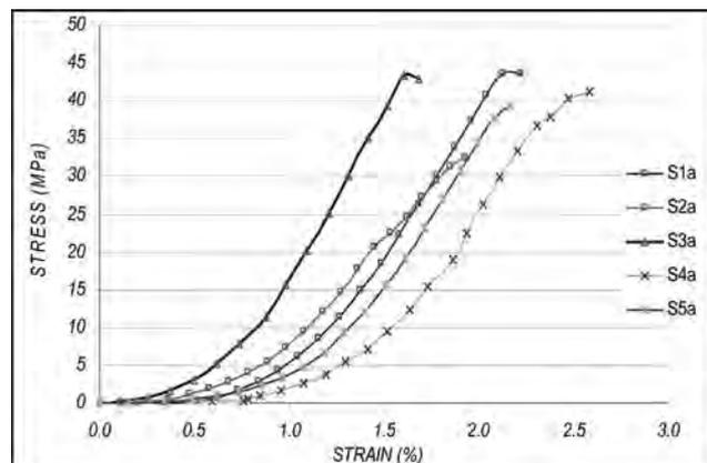
**Figure 6:** Stress-strain curve for sandstone tested under conventional testing machine.
