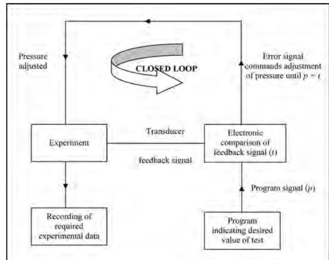
**Figure 3:** Principles of closed-circuit servo-controlled system (after Hudson *et al.*, 1971).
