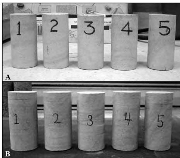
**Figure 4:** Sandstone samples for testing using (A) MaTest conventional compression testing machine and (B) Tinius Olsen servo-controlled testing machine.
