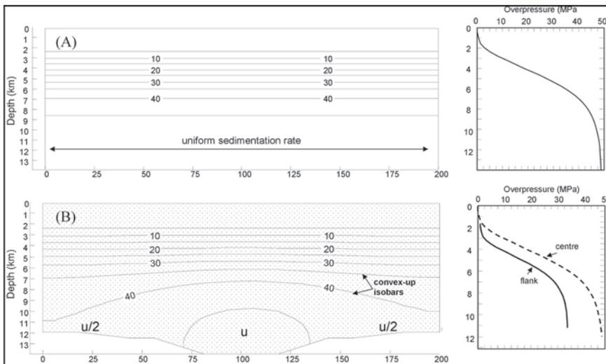
**Figure 14.** Influence of sedimentation rate on overpressure. A) If the sedimentation rate is uniform across the basin, the overpressure thus developed will be uniform all along the basin profile – i.e. straight contours. B) In this example, the sedimentation of the oldest unit on the flanks (Group M) is reduced to half that at the centre. This reduces the magnitude of overpressure on the margins; and the isobars assume a convex-upward shape.
