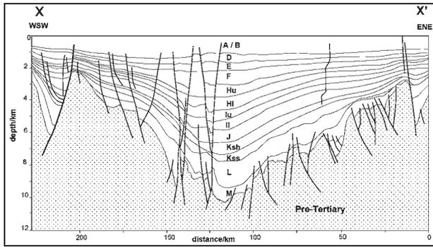
**Figure 3.** Line drawing of seismic section along XX' in Figure 1, showing the basin geometry and stratigraphy of the northern Malay Basin.
