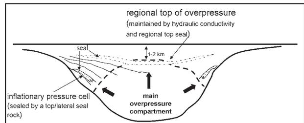
**Figure 17.** A schematic diagram of the Malay Basin, showing the relationship between the main basin overpressure compartment and secondary compartments (cells) on the flanks.
