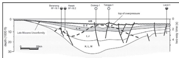
**Figure 2.** A profile across the Malay Basin from M Shariff Kader & Leslie (1995), depicting the general form of the overpressure cell in the basin centre. Note the convex-upward of the top-overpressure surface, cutting across stratigraphy towards the basin margins. The authors also observed a region of relatively shallow overpressure in the Beranang/Resak trend.
