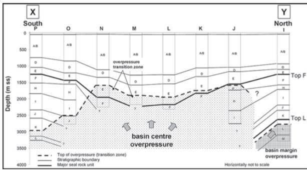
Figure 7. Line XY showing top of overpressure in relation to the stratigraphy in the key wells studied. (See Figure 6 for location).
