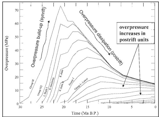
**Figure 12.** Pressure-depth plots for a central location, showing the changes in overpressure with time for each stratigraphic unit. The model assumes uniform sand-shale ratios for all rock units (0.25), and has 40 nodes in horizontal and vertical cells 1000 m thick.
