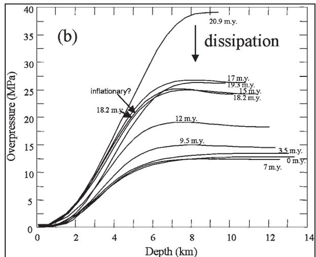
**Figure 13.** Overpressure-depth plot at key time steps during basin evolution, for a central location, showing the build-up and dissipation phases. During the latter phase, minor fluctuations in overpressure may occur.
