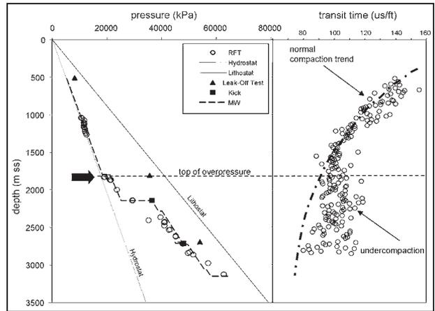
**Figure 5.** A pressure-depth plot in a well from the northern Malay Basin. Overpressure is detected at 1800 m where the pressure increases to the right of the hydrostat. Interval transit time from sonic log indicates undercompaction due to overpressure.
