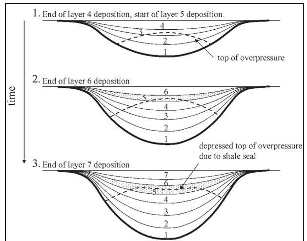
**Figure 16.** Schematic illustration of the development of a regional pressure seal (layer 5, representing Group F), which is responsible for the present-day depth to overpressure observed in the North Malay Basin.
