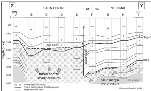
Figure 8. Line ZY showing top of overpressure in relation to the stratigraphy and structure of the basin. (See Figure 6 for location).
