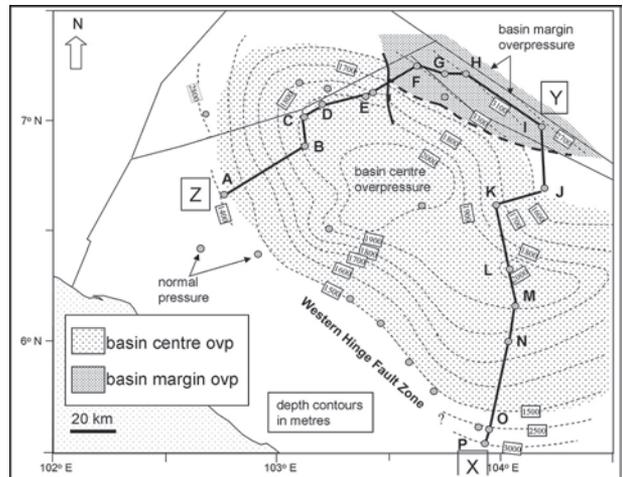
**Figure 6.** Map of the depth to the top of overpressure, Malay Basin, constructed based on pressure-depth plots in this study. Note that there are two overpressure compartments: a main one in the centre and a smaller one on the northeastern margin.
