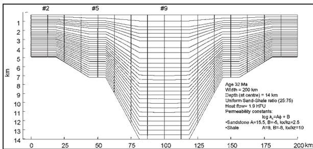
Figure 9. Idealised basin model for input in simulation, based on the cross section in Figure 3, intended to represent the Malay Basin. #2, #5 and #9 are pseudo-wells in the model, mentioned in later figures.
