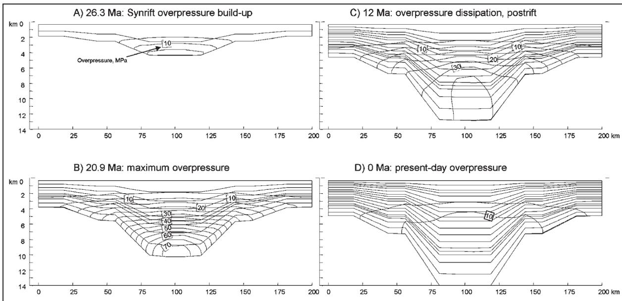
**Figure 10.** Snapshots of basin simulation at A) 26.3 Ma before present (BP), B) 20.9 Ma BP, C) 12 Ma BP, and D) 0 Ma BP. Note that 1) overpressure builds up as soon as first two layers of sediment have been deposited, 2) maximum overpressure is attained by 20.9 Ma BP at the end of the synrift phase (cf. Figure 11), and 3) overpressure starts to dissipate thereafter to present-day.
