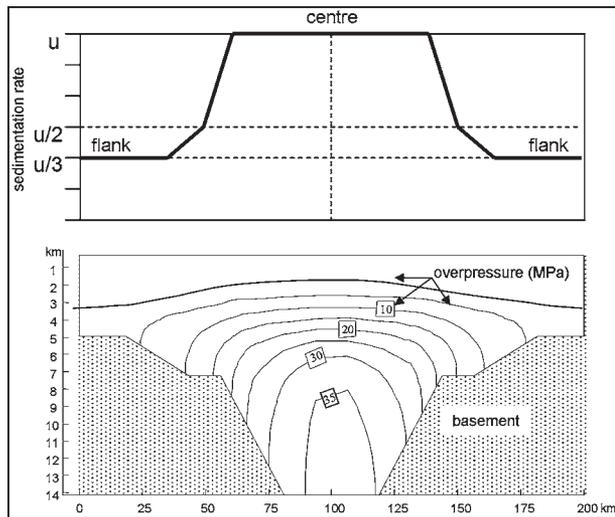
**Figure 15.** Influence of sedimentation rate on overpressure: this example has a varying sedimentation rate such that the rate of all the sedimentary units on the flanks is 1/3 of that at the centre. The resulting overpressure profile has a convex-upward shape.
