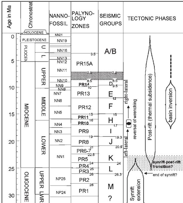
**Figure 4.** Stratigraphy of the Malay Basin and the corresponding tectonic phases.
