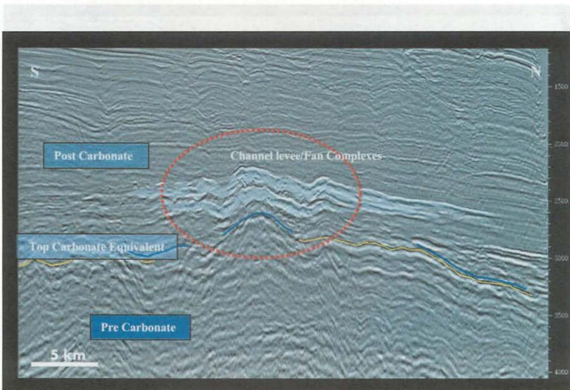
Figure 4. A seismic line across the proximal turbidite fans.
