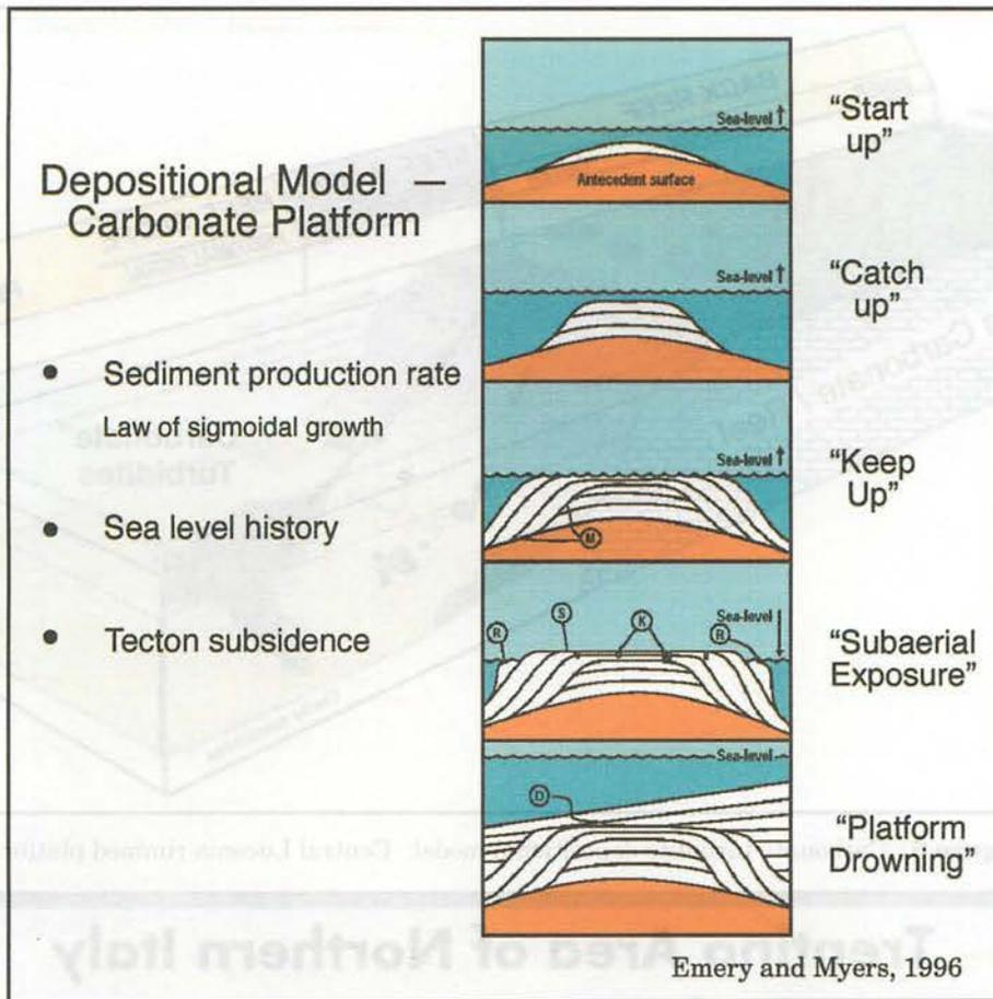
Figure 7. Schematic model for an isolated carbonate platform.
