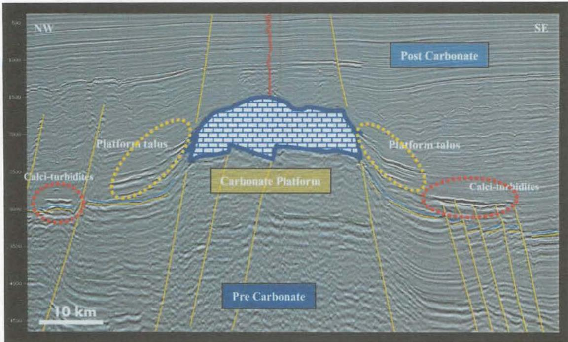
Figure 5. A seismic line across the carbonate high showing carbonate talus scree and turbidite fans.
