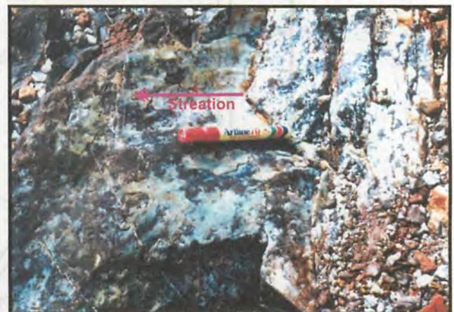
Figure 6. Striation on the shear plane, cutting the boudinage. Photo direction to NW.
