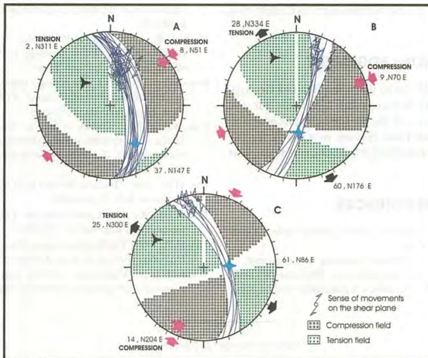
Figure 7. Paleostress and stress field responsible for the deformation of the serpentinite bodies in Felda Bukit Rokan Barat. (A) First period (D1), (B) Second period (D2), (C) Third period (D3).
