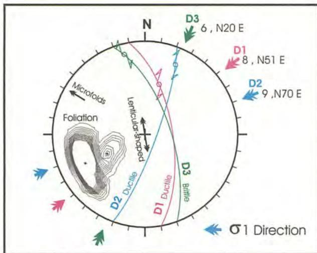
Figure 8. The structural elements of the serpentinite bodies and the direction of  $\sigma_1$  related to D1 (ductile), D2 (ductile) and D3 (brittle).
