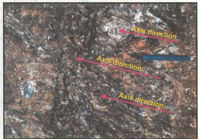
Figure 5. Microfolds within the shear zone (1st period). Photo direction to NE.
