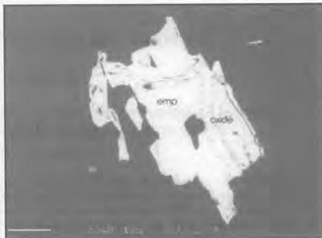
Figure 2. Backscattered electron image of emplectite (emp),  $\text{CuBiS}_2$ , from Bukit Panchor. The right hand part of the mineral is altered to a bismuth oxide mineral. Elemental composition for this mineral is given in Figure 3.
