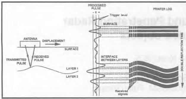
Figure 1. The reflected energy (signal) received displayed in the computer screen.
