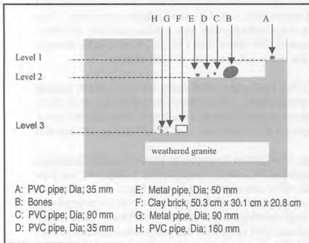
Figure 2. The cross section of the trench with relevant objects buried at different levels.
