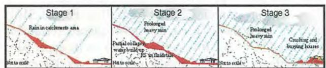
Figure 11. Mechanism of landslide.
