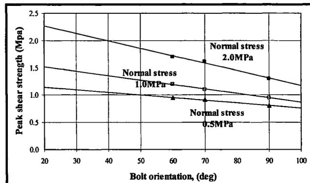
Figure 7. Peak shear strength versus bolt orientation at normal stress 0.5, 1.0 and 1.0 MPa.
