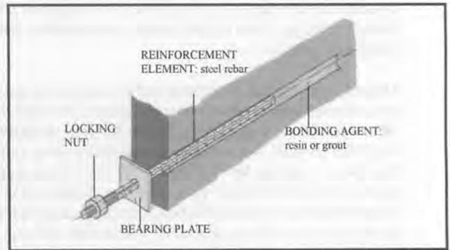
Figure 1. Full-bonded rock bolt (after Brady and Brown, 1985).
