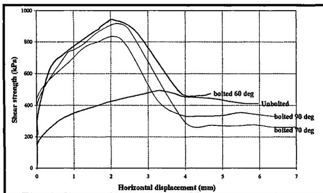
Figure 4. Shear strength of unbolted and bolted joint (90°, 70° and 60° bolt orientation) at normal stress 0.5 MPa.
