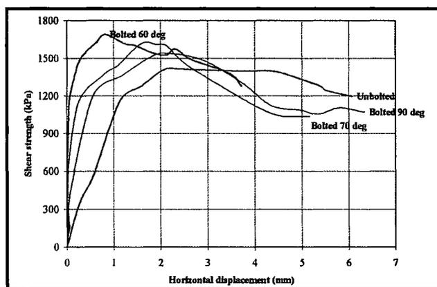
Figure 5. Shear strength of unbolted and bolted joint (90°, 70° and 60° bolt orientation) at normal stress 2.0 MPa.
