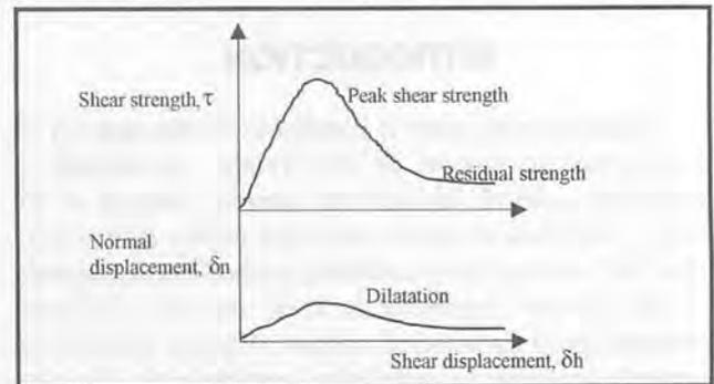
Figure 2. Shear strength and normal displacement versus shear displacement.
