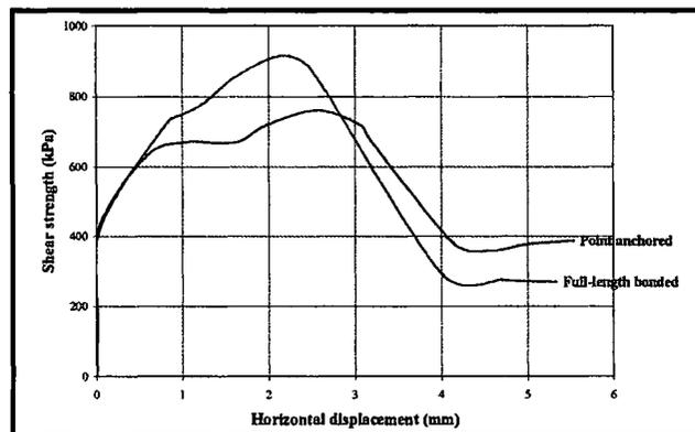
Figure 6. Shear strength of joint bolted with full-length bonded bolt and point-anchored bolt, at normal stress 0.5 MPa.
