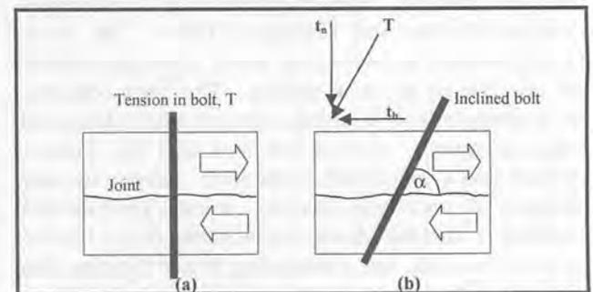
Figure 3. Rock bolt intersecting a joint, (a) perpendicular and (b) at angle  $\alpha$  to joint plane.
