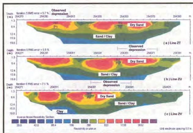
Figure 6. Examples of 2D resistivity imaging profiles conducted in the study area.
