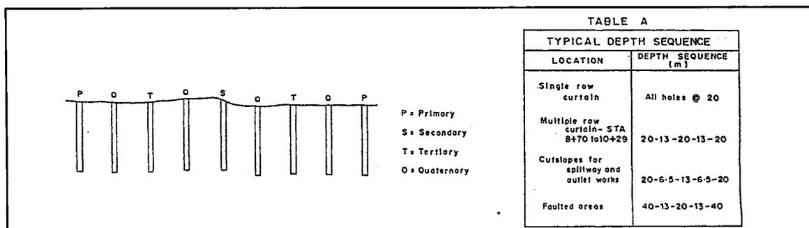
Figure 7. Grouting sequences.
