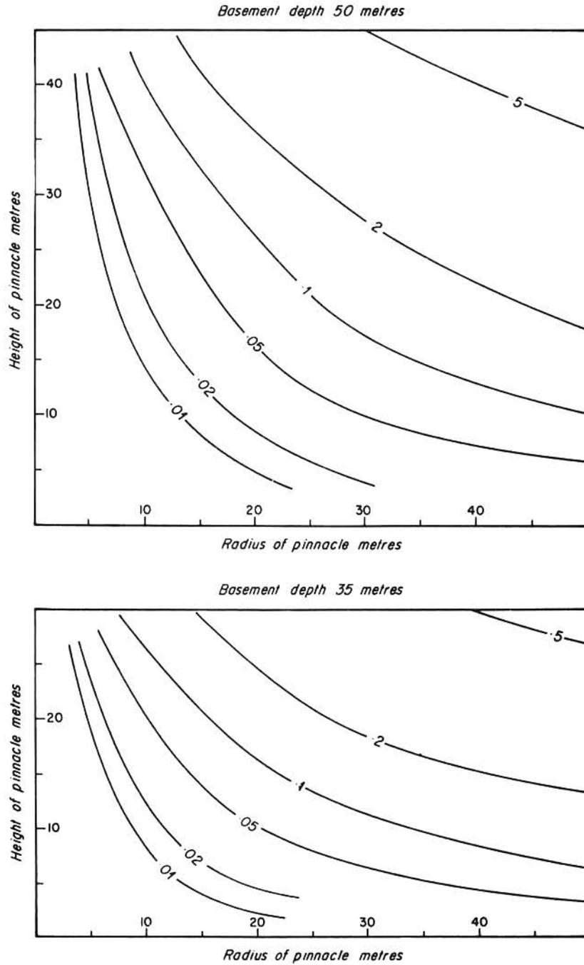
Fig. 1. Representation of gravity anomaly profiles over a pothole and a pinnacle modelled as vertical cylinders of anomalous density extending from the bedrock alluvium contact.
