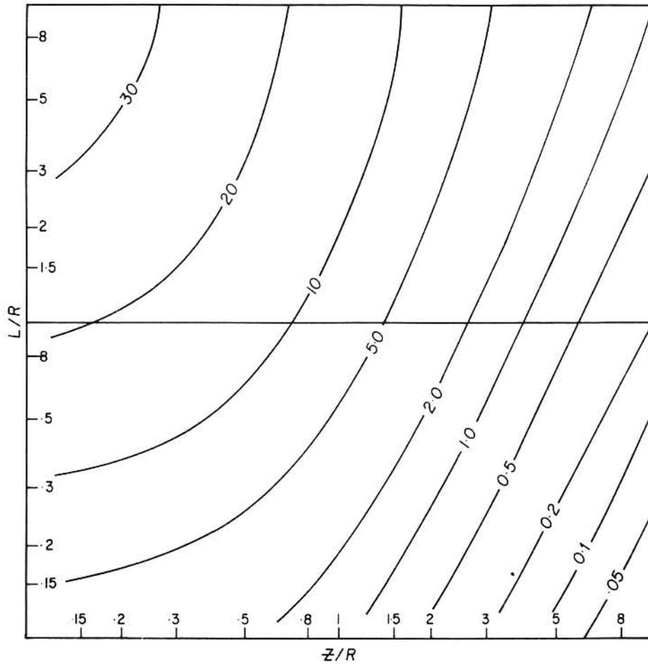
Fig. 3. Milligal contours of peak Bouguer anomaly amplitudes over pinnacles rising from basement depths of 10 and 20 metres. A 0.7 gm cc density contrast is assumed, for different density contrasts the amplitude is changed proportionately.
