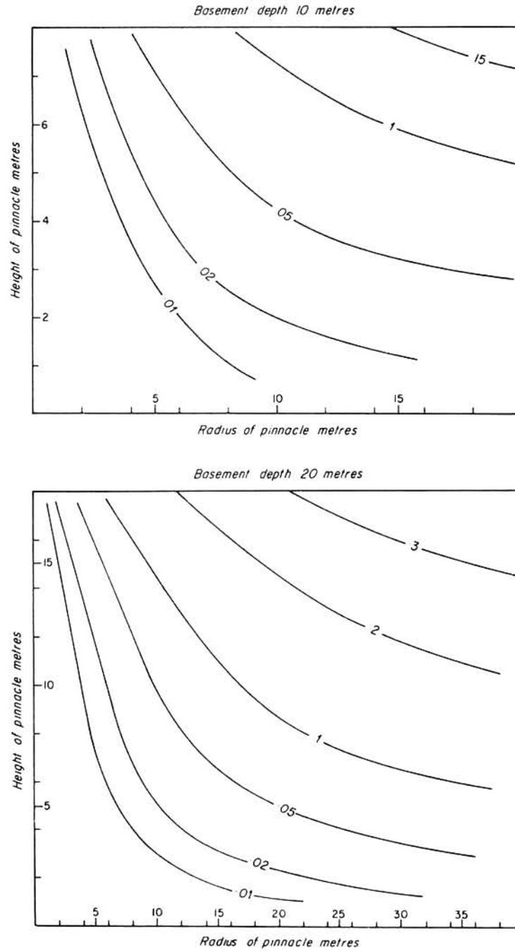
Fig 2 Milligal contours of peak Bouguer anomaly amplitudes over vertical cylinders. For explanation see text.
